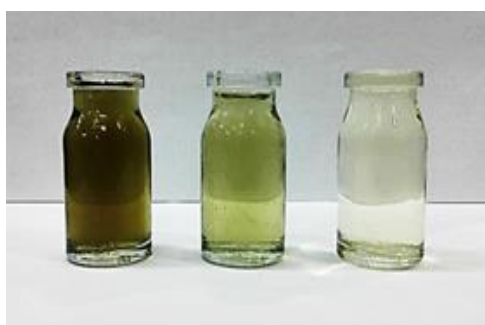
Fig. 16. The amount of decolorization of the real effluent sample from the textile wastewater prepared from the textile industry
