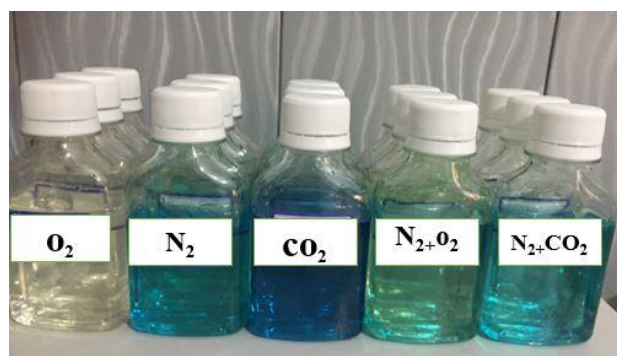
Fig. 9. Comparison of the color changes of Methylene Blue samples with the passage of time up to 20 minutes with the help of CO 2 , N 2 , O 2 gases
