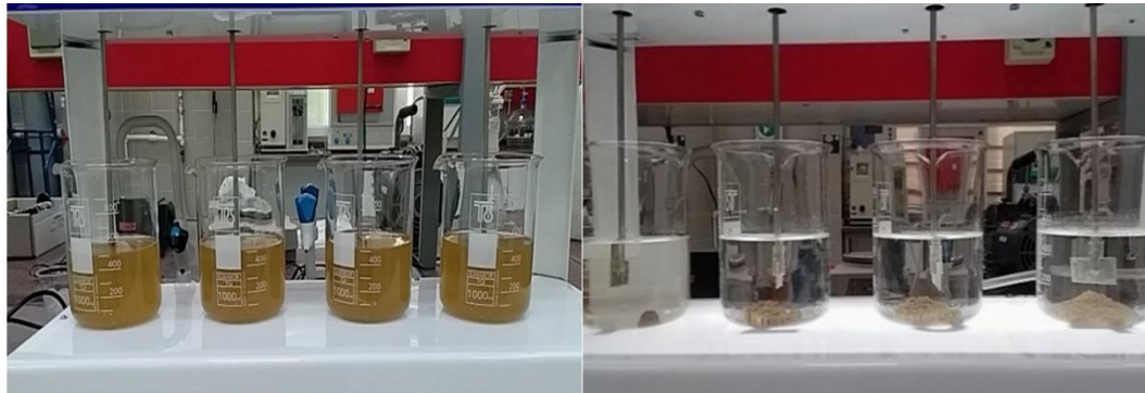
Fig. 2. Samples of 500 ml of wastewater before and after the Jar Test
