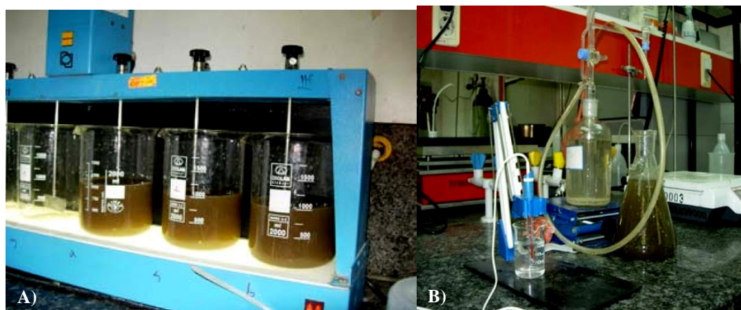
Fig. 3. Tests samples in laboratory Jar test Facilities, A) pH and B) temperature control
