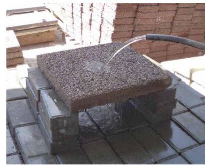
(A): Permeable pavement used in the project
