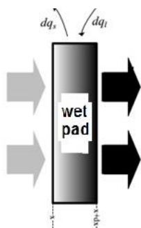
Fig. 6. Schematic of air flow across the width of the wet pad (He et al., 2014)
