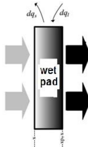
Fig. 2. Schematic of air flow across the width of the wet pad
