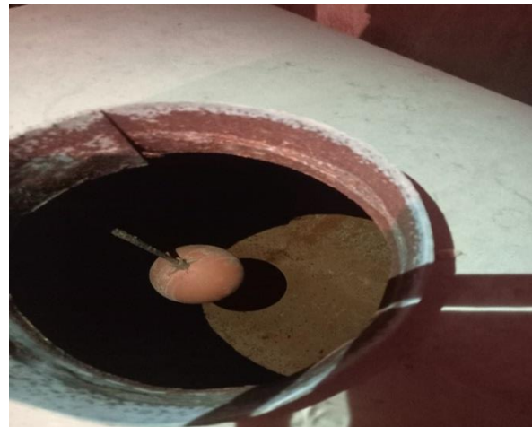
Fig. 8. Schematic of galvanized steel cistern with rust
