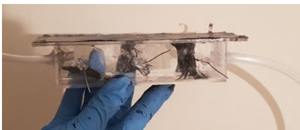
Fig. 1. Photo of the constructed microbial fuel cell
