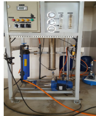
Fig. 1. View of: a) image of the device used in the experiments and b) schematic of the laboratory apparatus including: 1- tank with cooling system, 2- pump, 3- barometer, 4- carbon filter, 5- micron filter, 6- high pressure pump, 7- membrane chamber, 8- flowmeter, 9- refined flow, 10- concentrated excreted flow
