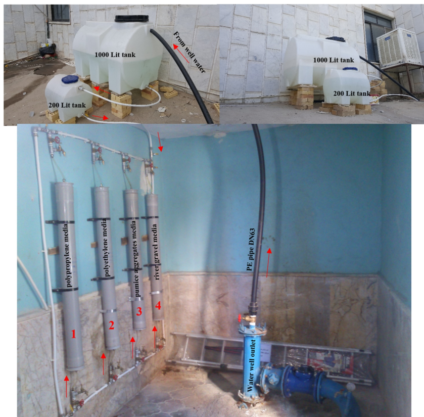
Fig. 1. Experimental pilot set-up in the nitrate contaminated well chamber
