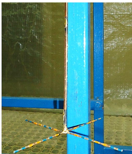
Fig. 3. Measuring annular jet flow thickness in the vertical shaft
