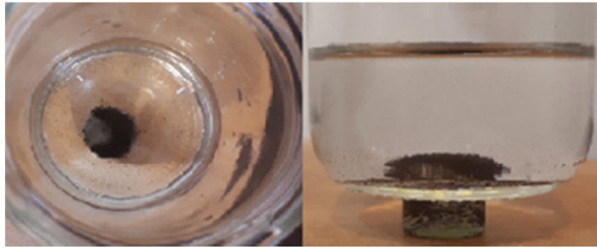
Fig. 13. Magnetic separation of T 88 F 6 G 6 nanocomposite
