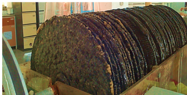
Fig. 2. The formation of attached biofilm (on discs) at the end of discontinuous operation cycle of the reactor
