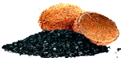
Fig. 3. Activated carbon from coconut skin
