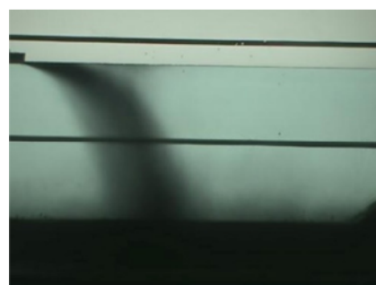
Fig 4. Averaged image of surface discharge in stagnant environment
