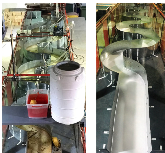
Fig. 1. Scheme of experimental flume and meandering channel
