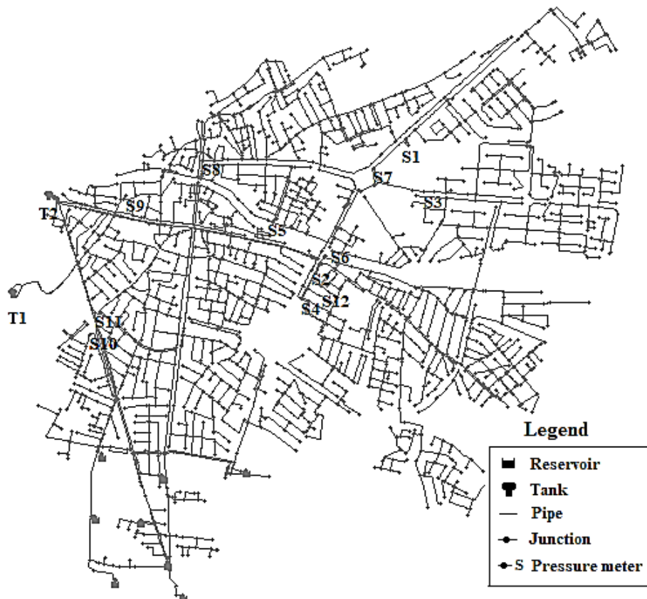
Fig. 2. Schematic of the Oshnaviyeh water distribution network
