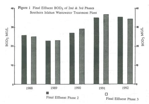
category of wastewater, because of the dying materials, usually enters into wastewater treatment plants separately. However at the Southern Isfahan Treatment Plant, this is not the case since the volume of domestic wastewater is higher than the textile industrial wastewater. Conversely, at Shahinshahr Treatment Plant, which has recently started recieving textile industry wastewter from northern Isfahan, a continuous and separate network is used.
