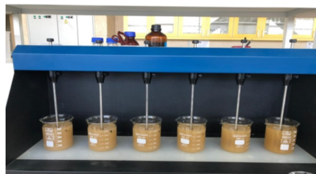
Fig. 1. A view of the Jar test to determine the optimum coagulant in the turbidity of 500 NTU
